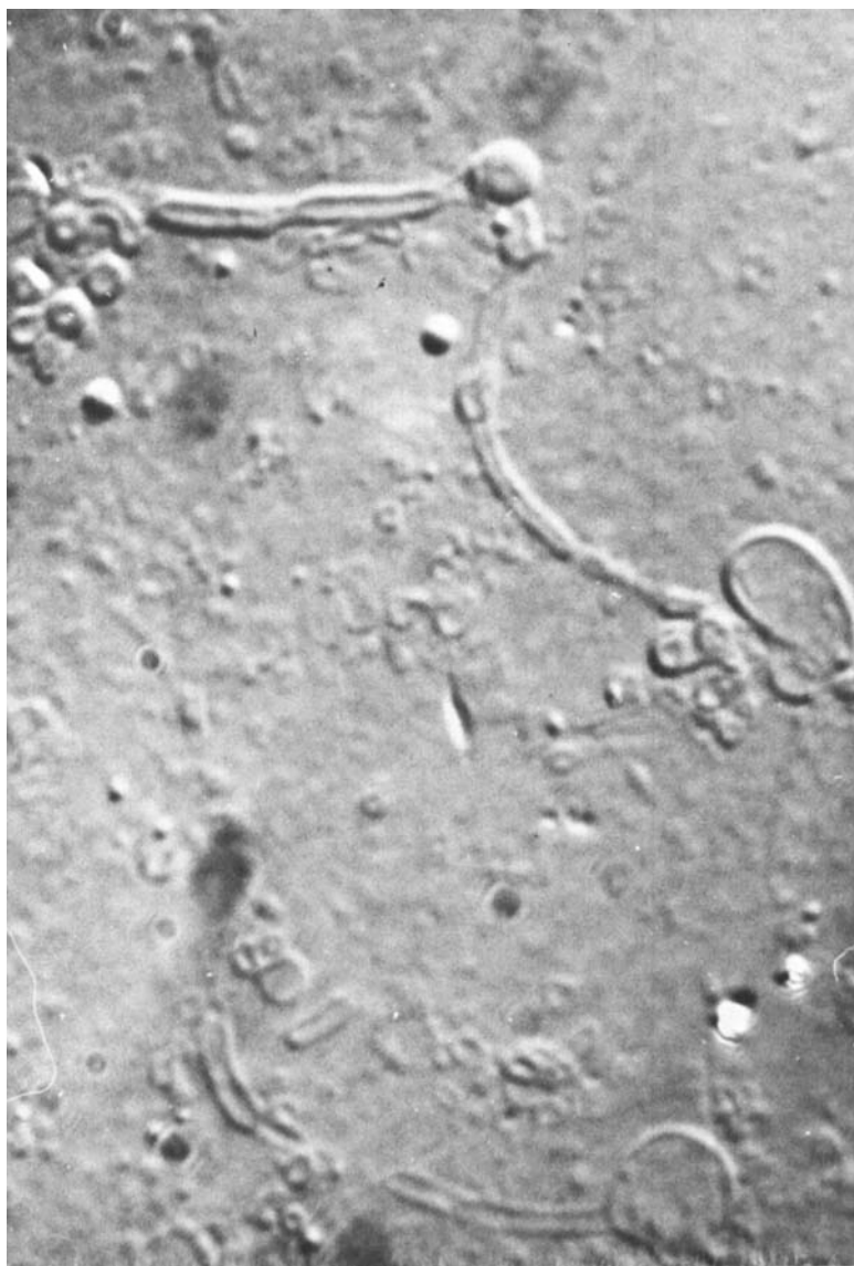
FIGURE 5 Nomarski Differential Interference Micrograph of tubules in aqueous mixed surfactant system. 4,100x
