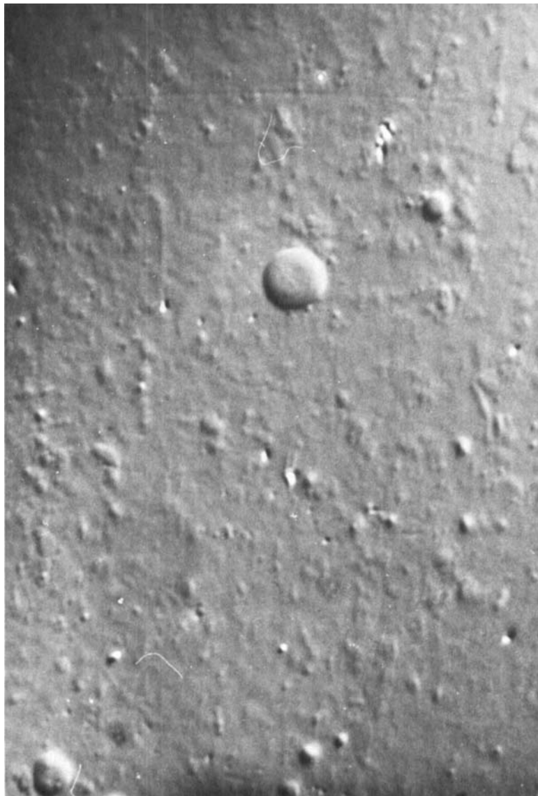
FIGURE 4 Nomarski Differential Interference Micrograph of vesicles in aqueous mixed surfactant system. 4,100x
